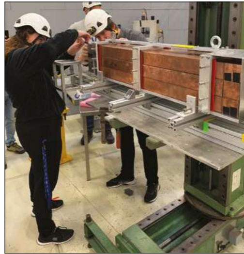
Saturation specific ALICE's new high-granularity forward calorimeter is designed to study gluon saturation.
